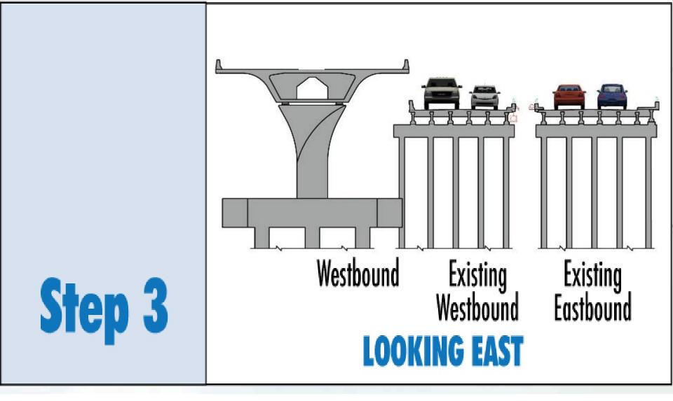
The remainder of the westbound bridge is built. Once the bridge is complete, temporary barriers are placed on the structure for the temporary traffic configuration.
