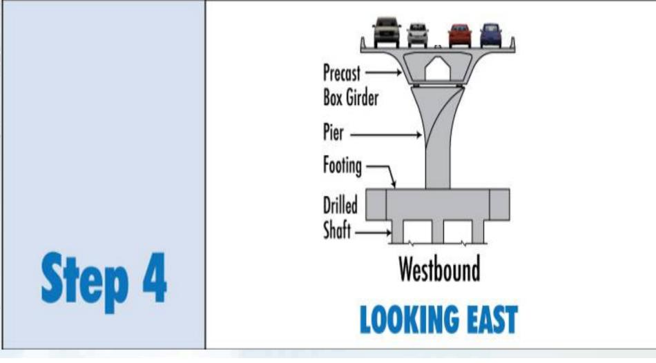
All traffic, two lanes in each direction, is moved to the new westbound bridge. The wider deck width allows for four lanes of traffic to be accommodated temporarily. Utilities are completely relocated to the new westbound bridge. Both the existing eastbound and westbound bridges are removed.
